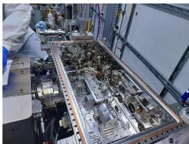
Figure 3: Mirror system working in UHV regime and partial pressure of oxygen to reduce the carbon contamination.
