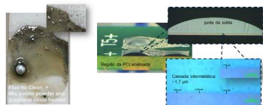
Fig. 2. a) Powder added to the heated flux, b) Metallographic analysis. Graphene oxide agglomerates on the solder joint surface. Intermetallic \sim 1,7\mu\text{m} .
